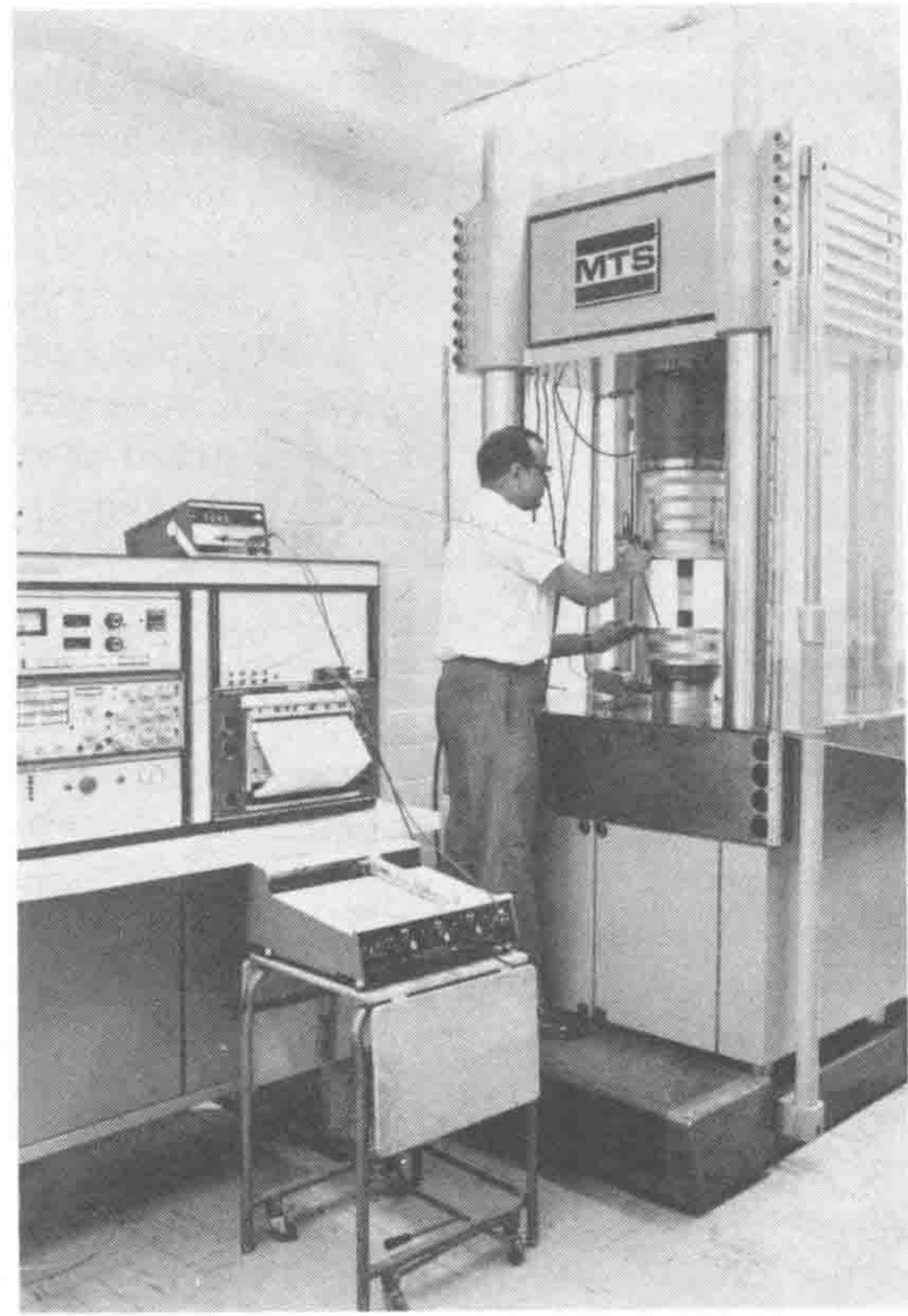
Fig. 4. 2000 kN Capacity testing equipment.
